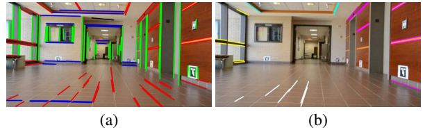
Fig. 5. Structural features in the corridor scenario: (a) three orthogonal VPs detection result; (b) four coplanar line matches which corresponding to different 3D planes are determined by one horizontal VP, and marked with respective colors (only one image of the matched image pair is shown).
