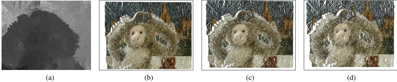
Fig. 4. (a) Corresponding depth map of recovered view in Fig. 3(d) (near=dark, far=light); (b)-(d) Three re-projected images on input images.
