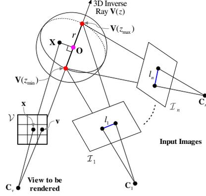
**Fig. 2.** Measure of new matches of neighboring pixels around seed points. Based on the piecewise smooth assumption in the spatial domain, both valid depth search range and depth sampling number are determined.
