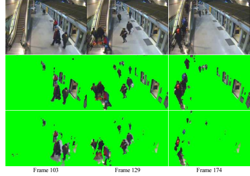
Figure 8. Results on a metro video with a moving escalator (first row: original images; 2nd row: our method; 3rd row: MoG method).
