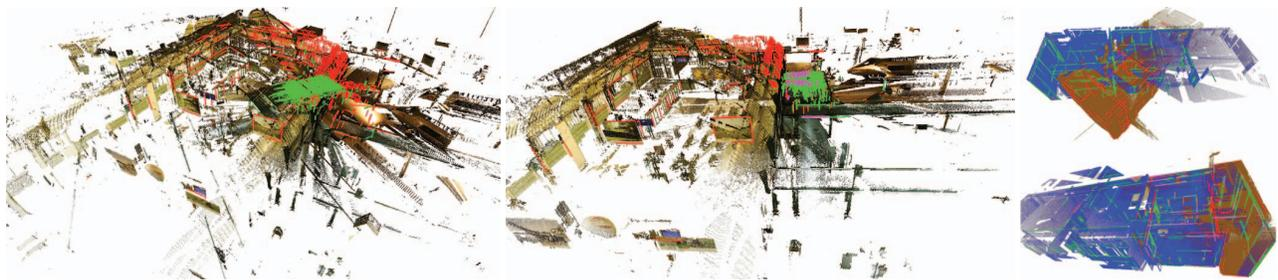
**Fig. 1.** Line matching results of two pairs of scans (Left: before matching, Middle: after matching, Right: top before matching and bottom after matching): *Red* lines related to first scan, *green* lines related to second scan. Matched lines are shown in *purple*.
