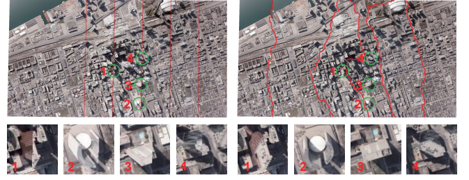
Fig. 3. An example of optimal seamline detection for parallax removal: overlapped edges (Left) and optimal seamlines (Right).
