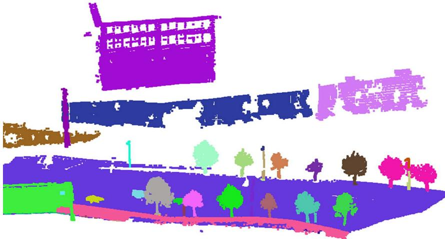
(b) the segmentation result after post-processing for the region II from the point cloud set  $S_2$ .**Figure 7.** The segmentation results before and after post-processing for the region II from the point cloud set  $S_2$ .**Table 5.** The comparison results between the classification of original P-Linkage segmentation and the classification based on the segmentation after post-processing for 3 testing point clouds.
