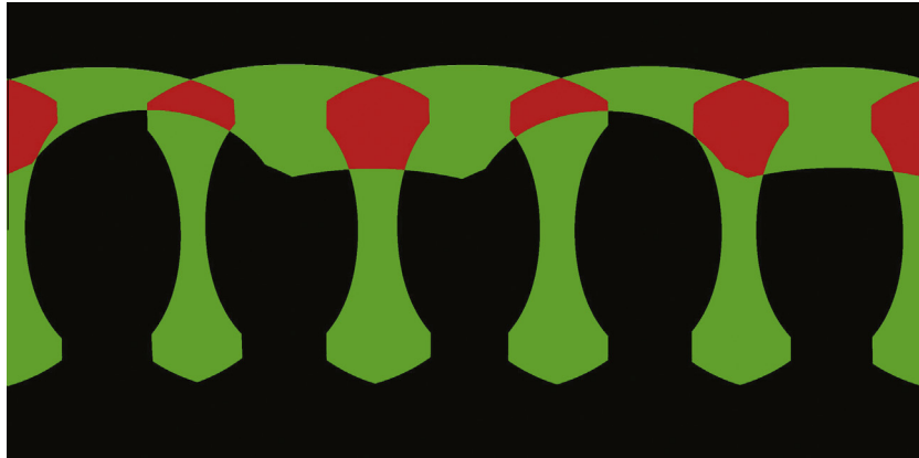
Fig. 8. The image overlap regions of six geometrically aligned and warped images in the 360° street-view panoramic view where the black, the green and the red represent the no-overlapped, two-overlapped, multi-overlapped image regions, respectively. (For interpretation of the references to color in this figure legend, the reader is referred to the web version of this article.)
