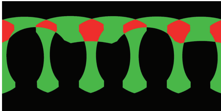
Figure 9. The image overlap regions of six geometrically aligned and warped images in the 360° street-view panoramic view where the black, the green and the red stand for the no-overlapped, two-overlapped, multi-overlapped image regions, respectively.
